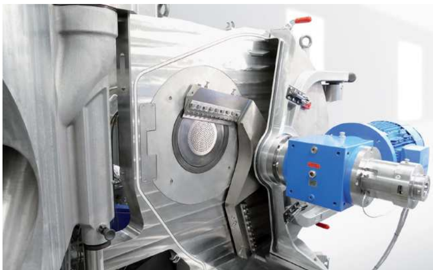
The redesigned Coperion EGR eccentric pelletizing system achieves higher compound quality and significant energy savings in the manufacture of temperature- and shear-sensitive plastics (Photo: Coperion, Stuttgart Germany)
